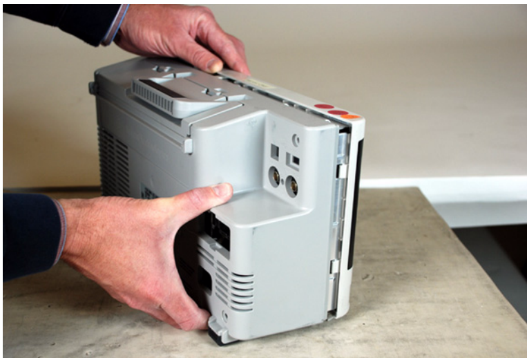
Figure 23 Removing bucket assembly
