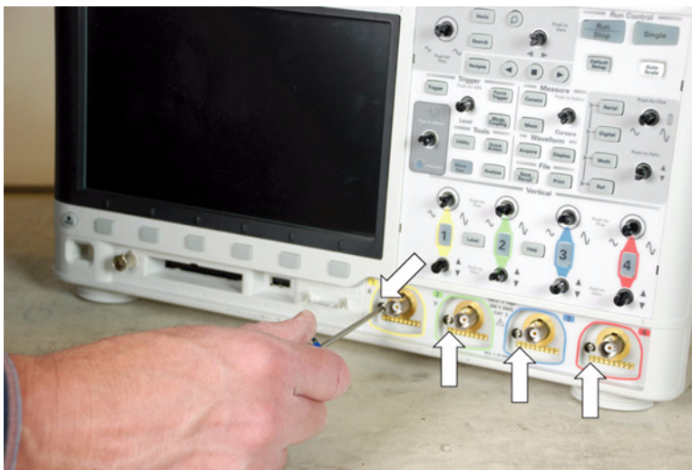
Figure 37 Removing the T6 screws (4 channel version)
