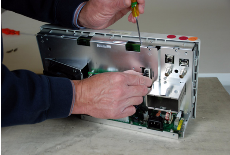
Figure 33 Disconnecting the interboard supply cable from the acquisition board
