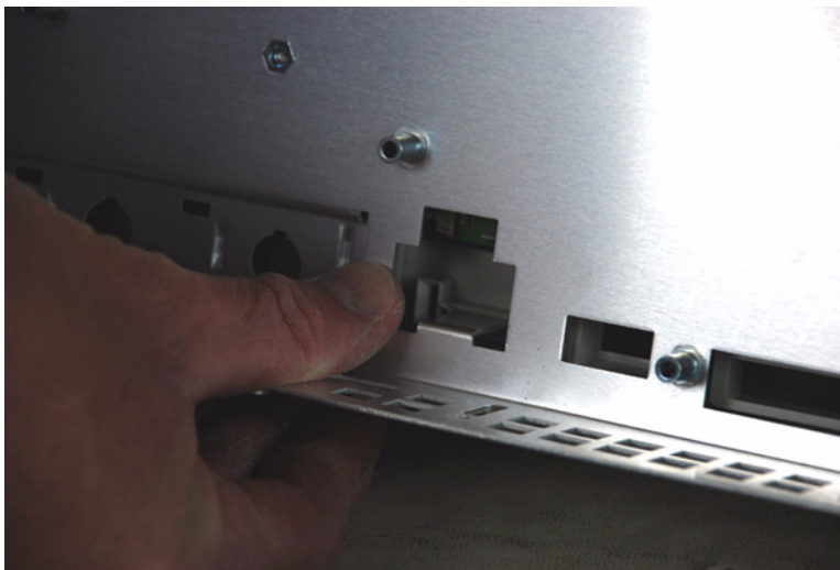
Figure 44 HINT: When reinstalling bezel, align ground terminal first
